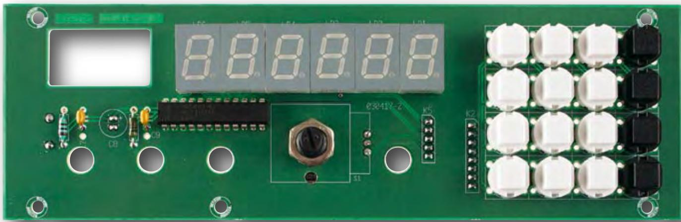
nection leads straight onto the board). The voltage regulators (IC5 and IC7) are also found here. These should be provided with a heatsink, otherwise they could overheat when the case is screwed shut. On the display board the following components are mounted on the underside of the board: the rotary encoder S1 (so the spindle sticks out through the front), the headers (if required) for K2, K5 and the supply, and electrolytic capacitor C8.
