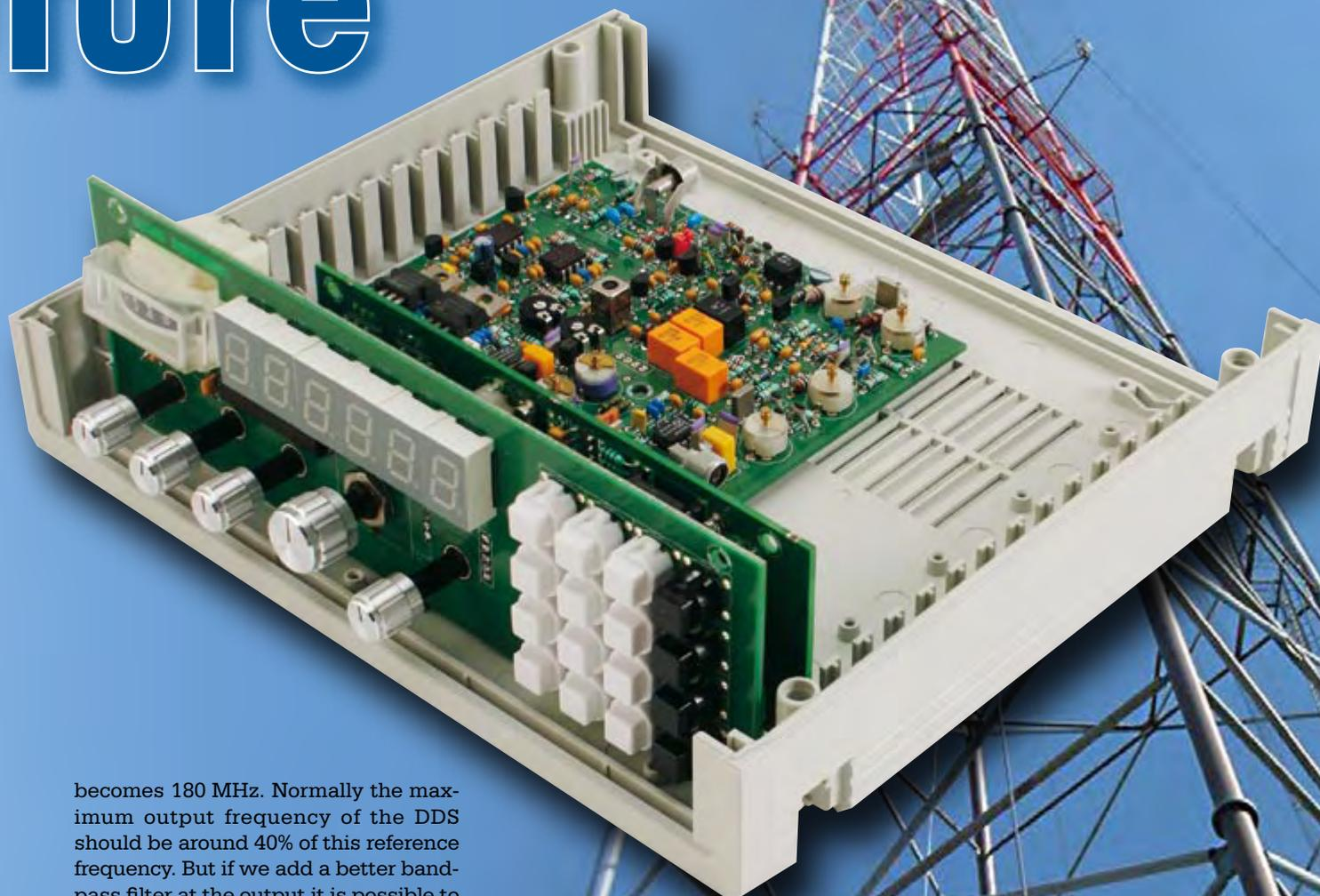
becomes 180 MHz. Normally the maximum output frequency of the DDS should be around 40% of this reference frequency. But if we add a better band-pass filter at the output it is possible to increase this figure somewhat.
